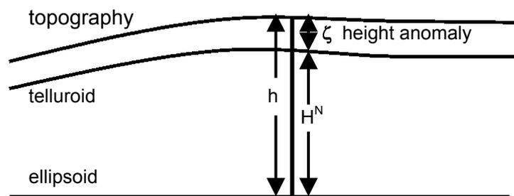
**Figure 2.2 Relationship between telluroid and ellipsoid.**
