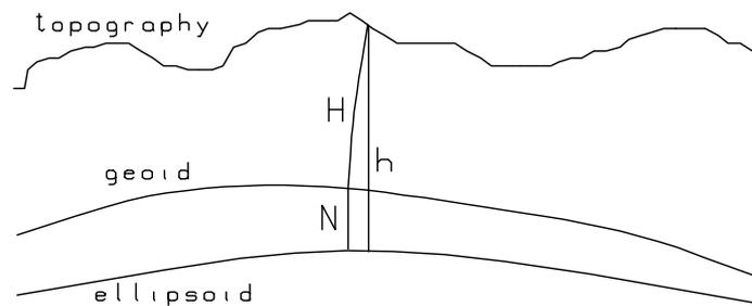
**Figure 2.1 Relationship between geoid and ellipsoid.**
