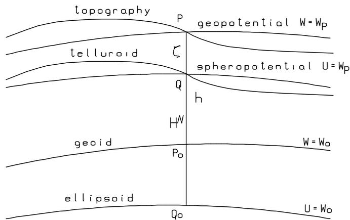
**Figure 2.4 The relationship between geopotential at ground surface and spheropotential at telluroid.**
